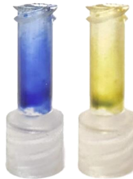
Fig. 2. Example of initial 3D printed connector with ammonia indicator before and after exposure.
